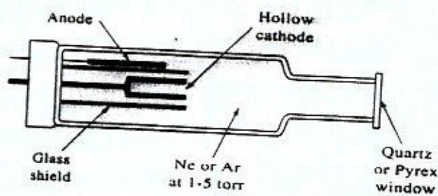
of cathode rays. These positive ions, bombard the cathode with high energy and sputter off the metal atoms. These metal atoms are excited to higher electronic levels by continuous collisions with high energy gas ions. When the electrons return to the ground state, the characteristic resonance line is emitted alongwith some other lines. This characteristic resonance line is absorbed by test element and its absorption is measured.
