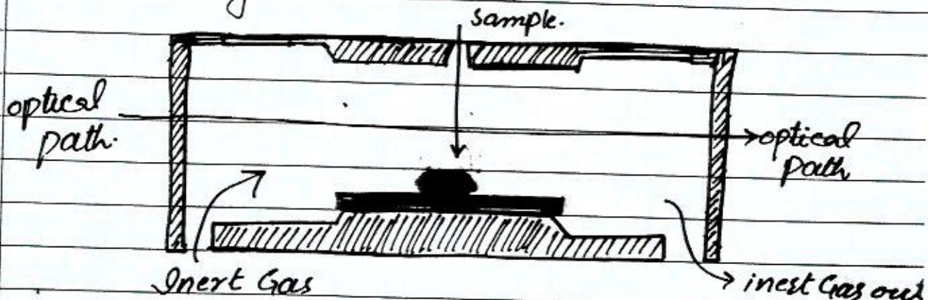
Samples of between 5-50 μL are injected into the graphite tube through a small hole at the top of tube. Atomization is achieved in three stages. In the first stage, the sample is dried to a solid residue using a current that raises the temperature of tube to about 110°C. In the
