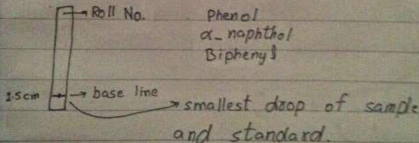
First of all, about 0.1% solution of sample is prepared in a suitable solvent then a thin pencil line is drawn across the plate, a few centimeters from the bottom (2 cm). Now the
